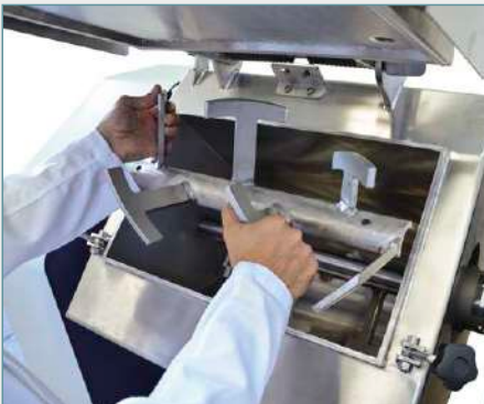
B026-05N Detail of the detachable mixing shaft with blades
