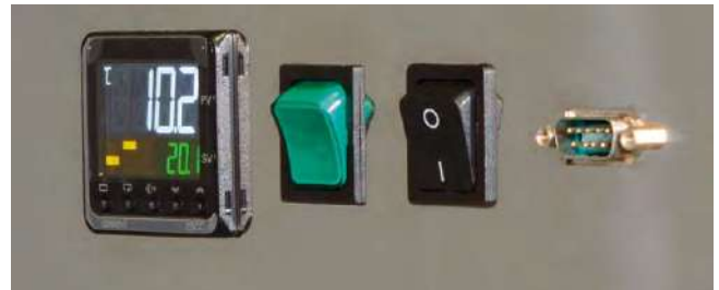
Cabinet switches and temperature controllers
