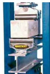
Flexure on concrete
