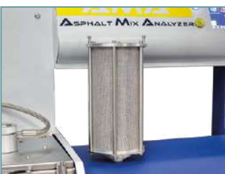
Integrated balance for automatic weight record
