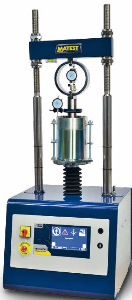
S212M with accessories for CBR test
