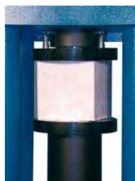
Compression on concrete
