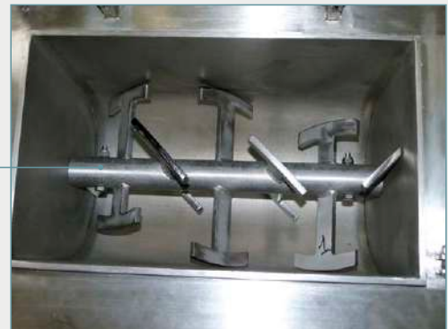
Detail: mixing shaft with helical blades
