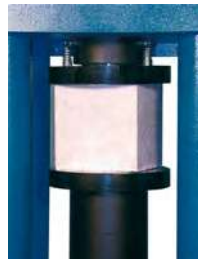
Compression on concrete
