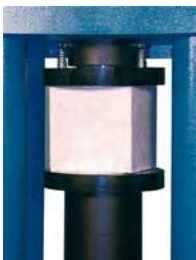
Compression on concrete
