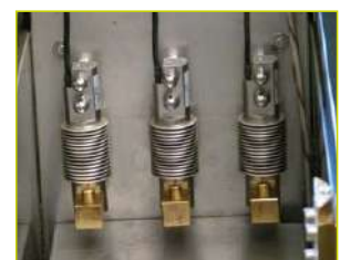
Detail: 3 load cells 500 N
