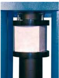
Compression on concrete
